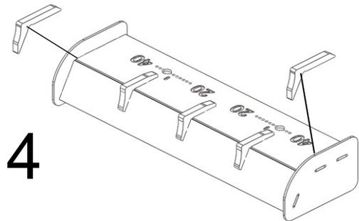
Place and glue (CA glue) the side support ribs (2 pieces) on bottom side of the flaps (making sure the support ribs are contacting the end plate)
