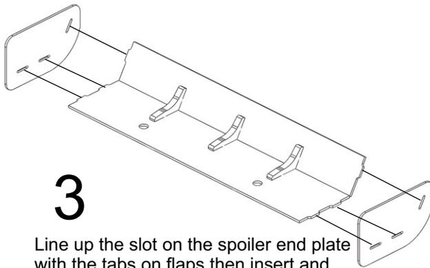
Line up the slot on the spoiler end plate with the tabs on flaps then insert and connect them together
