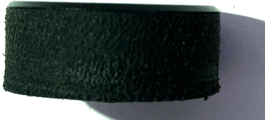
It is possible that a burr of the injection point remains on the inside of the sidewall. This can compromise the proper functioning of the part since it will not be continuously supported on the sidewall of the tire.
